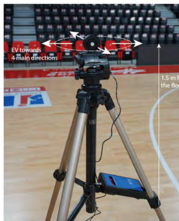
Vertical illuminance (EV) measurement
