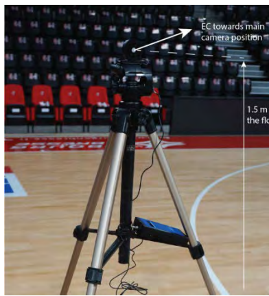
Main camera illuminance (EC) measurement
